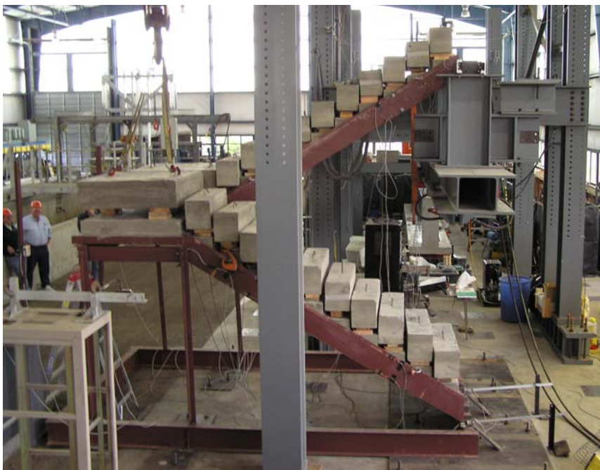
Fig. 6a – Prefabricated steel stair tests (Higgins 2009).
